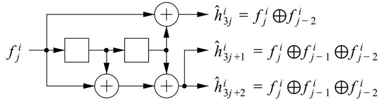
**Figure 3-8: Encoder for Rate 1/3 Mother Convolutional Encoder**
