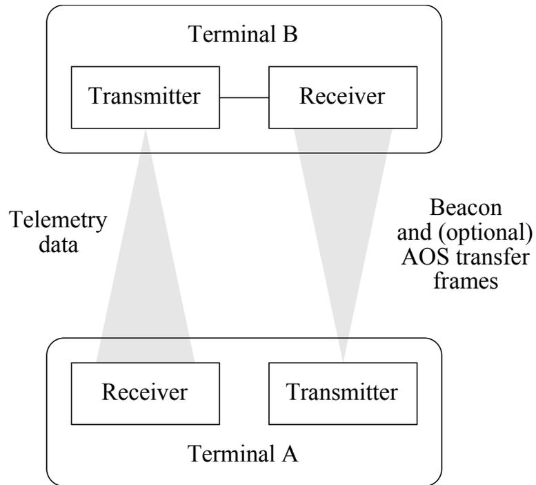
**Figure 2-2: Overall Architecture of the Optical Communications System**
