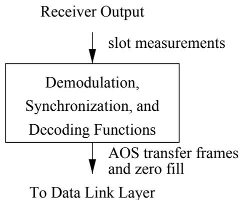
**Figure 2-6: Internal Organization of the AOS Transfer frame Signaling at the Receiving End**
