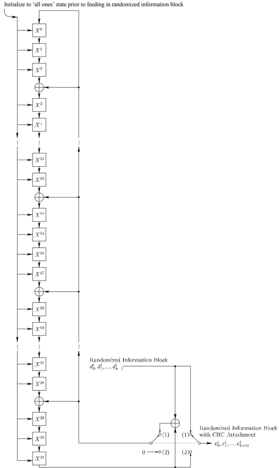
**Figure 3-5: Shift Register Implementation of CRC Attachment**
