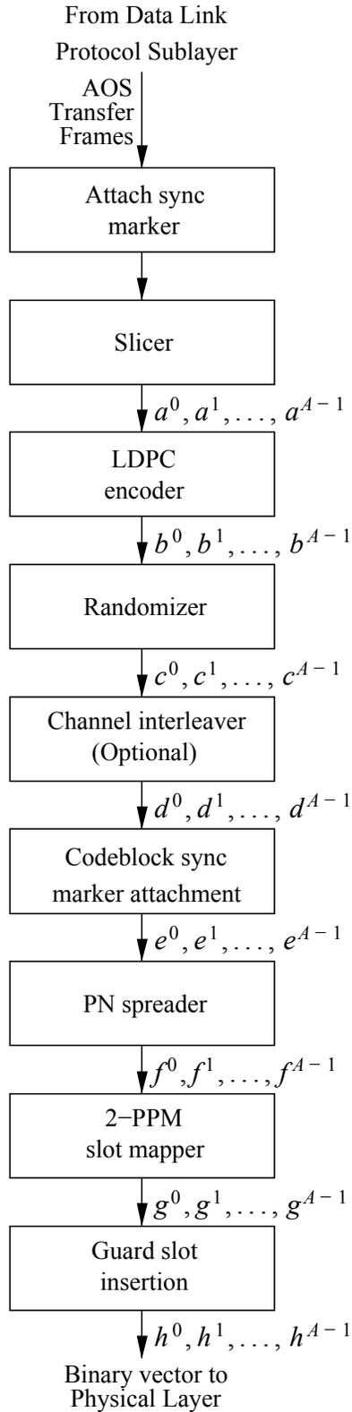
**Figure 4-1: Functional Diagram for AOS Transfer Frame Signaling**
