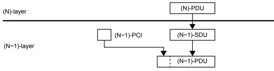
**Figure 1-2: Relationship between PDU, SDU, and PCI**
