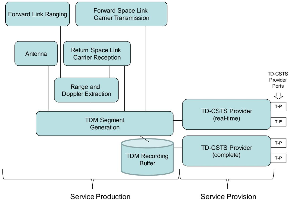
**Figure 2-1: Production and Provision of Tracking Data Cross Support Transfer Services**
