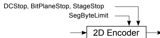
Figure 2-2: Compressor Quality and Rate Control
