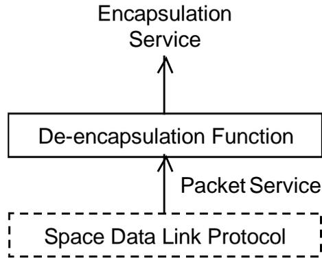
**Figure 4-4: Internal Organization of Encapsulation Service (Receiving End)**
