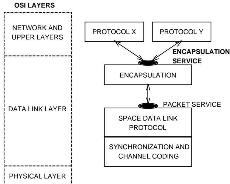
**Figure 2-1: Concept of Encapsulation Service**
