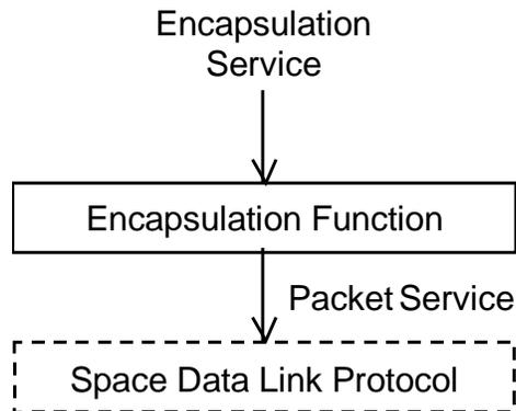
**Figure 4-3: Internal Organization of Encapsulation Service (Sending End)**
