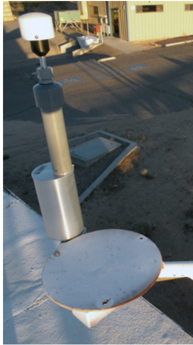
Figure A-4: Particle Profiler Deployed at the NASA/JPL Goldstone, CA Facility
