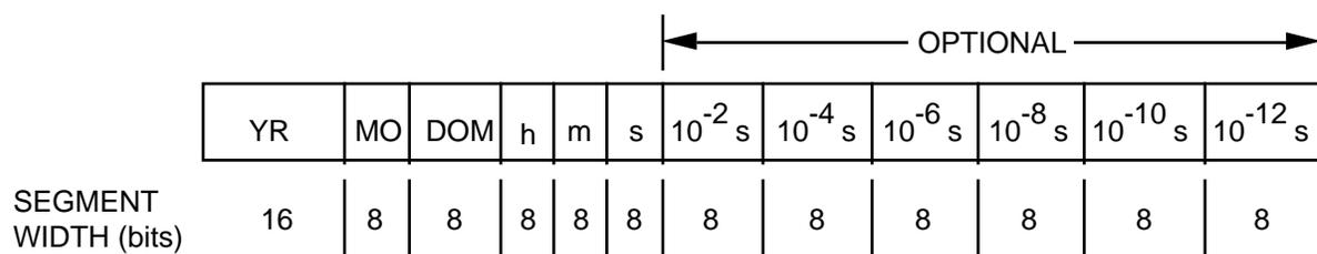
The year A.D. segment (YR) requires 16 bits for proper representation of the decimal year. All other segments require 8 bits for proper representation. The month (MO) and day of month (DOM) segments are present when the calendar variation flag (bit 4 of the P-field) is set to zero.
