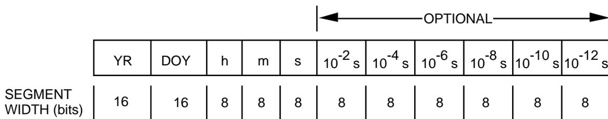
This variation of the CCS time code substitutes day of year (DOY) in place of the month (MO) and day of month (DOM) segments. The day of year segment must be 16 bits long (all segments must be multiples of 8 bits). The four most significant bits of this segment are not used and are set to zero. The day of year segment is present when the calendar variation flag (bit 4 of the P-field) is set to a value of one. The year A.D. segment is 16 bits in length.
