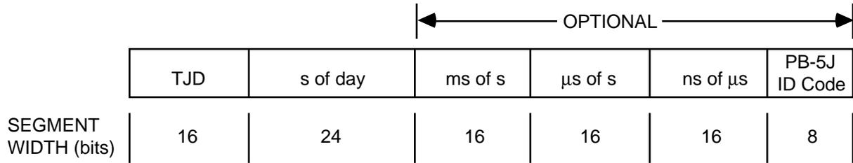
Fill bits have been added in the most significant position of each segment to ensure that the segments end on octet boundaries.
