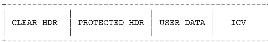
Figure 3-1: SCPS-SP Protocol Data Unit
