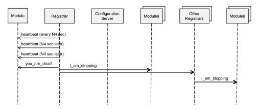
**Figure 5-4: Imputed Module Failure**
