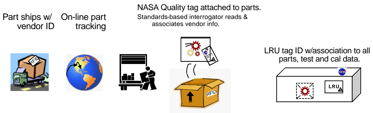
Figure 3-2: RFID Ground-to-Line Replacement Unit Concept
