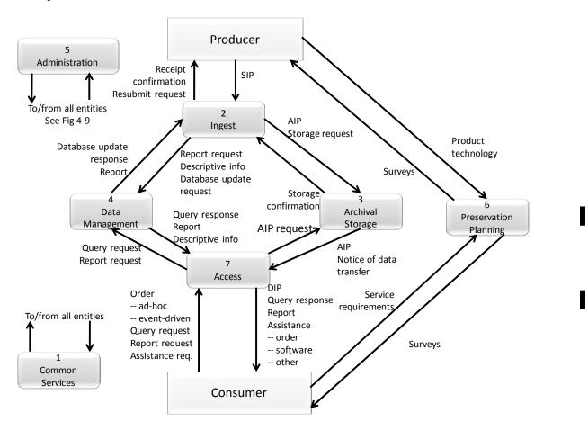
Figure 4-8: OAIS Data Flow Diagram
