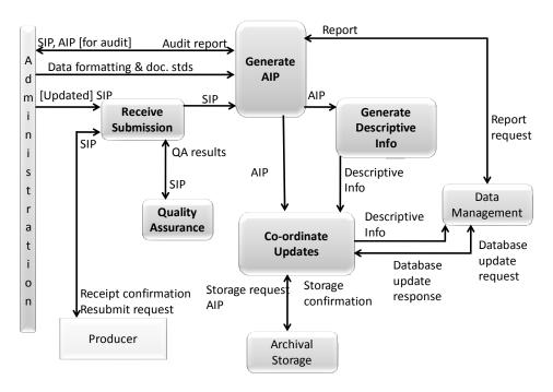
Figure 4-2: Functions of the Ingest Functional Entity
