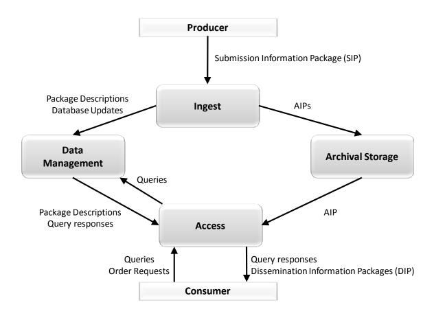
Figure 4-26: High-Level Data Flows in an OAIS
